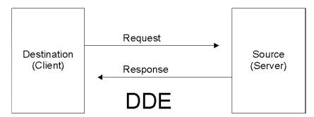
The Destination (Client) sends a Request to the Source (Server). The Source (Server) sends a Response to the Destination (Client).
